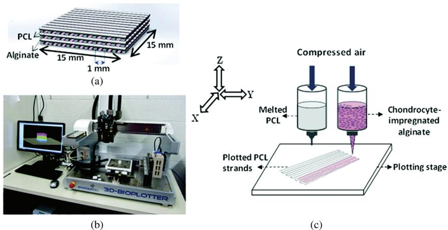
Fig. 2. Design and 3D bioprinting of hybrid constructs with structural and biological features. (a) Schematic of designed 3D hybrid construct with alternating strands of polycaprolactone (PCL) and chondrocyte-impregnated alginate in each layer, (b) 3D bioplotter system employed for biofabrication of designed hybrid constructs, and (c) hybrid biofabrication using pneumatic dispenser heads.<sup>30</sup>
