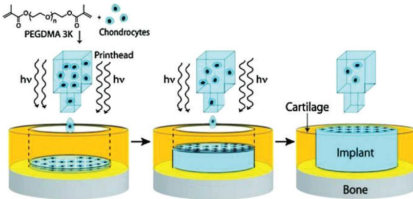
Fig. 1. Schematic of bioprinting cartilage with simultaneous photopolymerization process. PEGDMA, poly (ethylene glycol) dimethacrylate; hv, UV light energy.<sup>24</sup>
